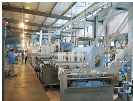
日产70吨高强低伸型瓶片纺涤纶后处理设备 70TPD flakes spinning draw-off equipment for high tenacity low elongation fiber
