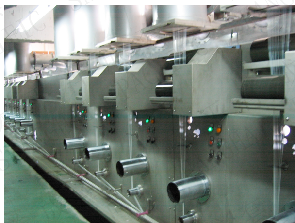
采用油轮双面上油，无网络生头器的卷绕墙 Two side finishing with oil wheeler, draw-off wall without net take-up
