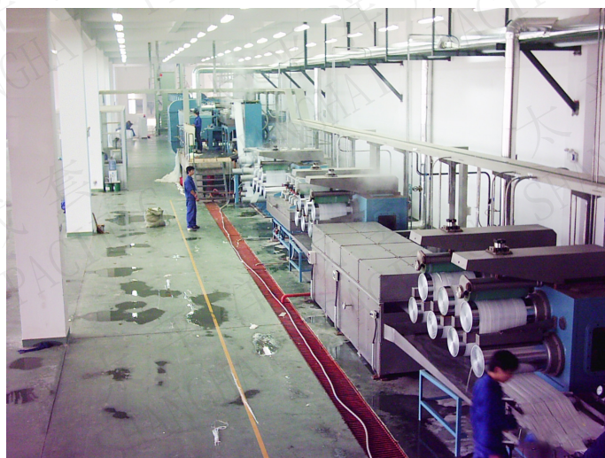
双组份LPET/PET复合涤纶短纤维生产线 Bi-components LPET/PET composite PSF production line
