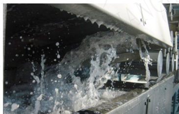
涌渍式牵伸水浴槽 可以将丝束的牵伸点精确地控制在水浴槽中 Immersion draw bath the draw point of the tow will be controlled precisely in the immersion bath
