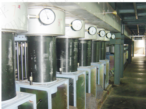
半敞开式环吹风，低阻尼外环吹，汽缸升降，有特殊结构可产生不对称冷却吹风的装置 Semi-open quench, low damping quench from outside Cylinder up and down with special structure device producing unsymmetrical cooling blow
