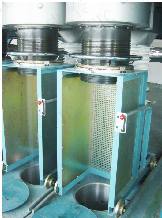
半敞开式外环吹 semi-open quenching from outside
