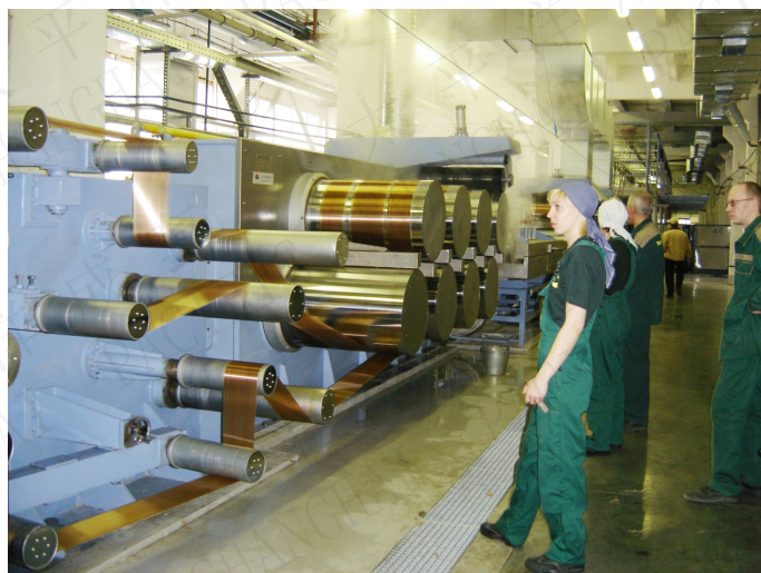
三维中空/普棉瓶片纺涤纶短纤维生产线(俄罗斯工厂现场) Flakes spinning PSF production line for 3 dimensional crimped hollow/solid cotton fiber Plant site in Russia
