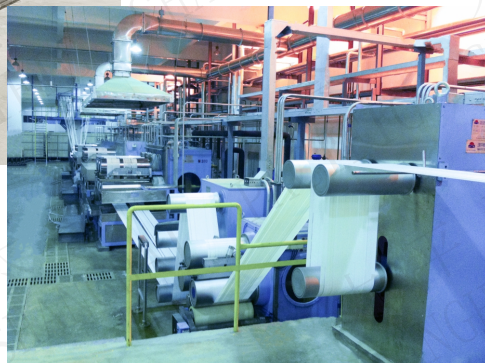
复合纺后处理联合机 Composite Fiber Draw Line
